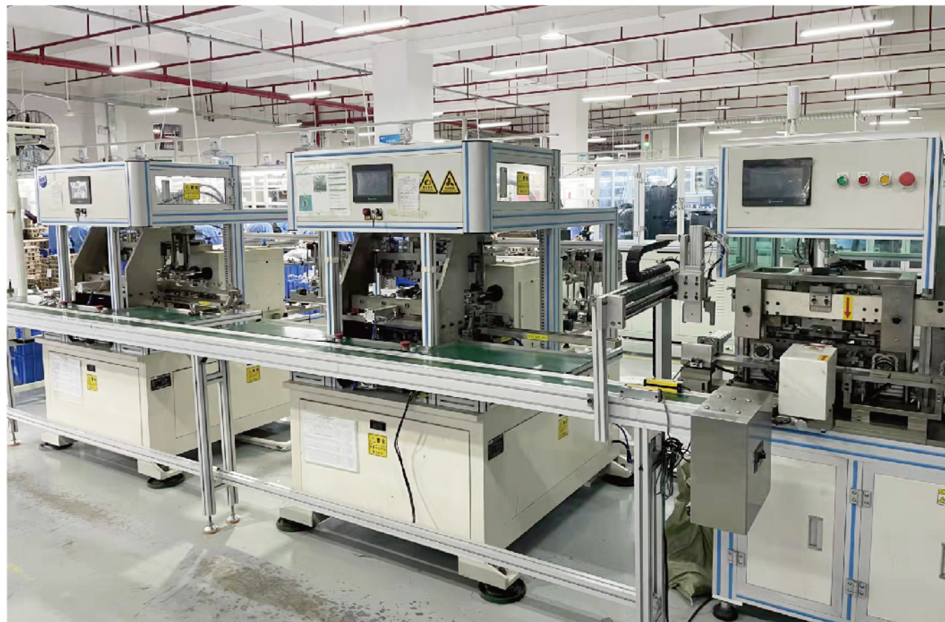
自动定子入槽机以及自动绕线机 /Automatic stator slotting machine and automatic winding machine
